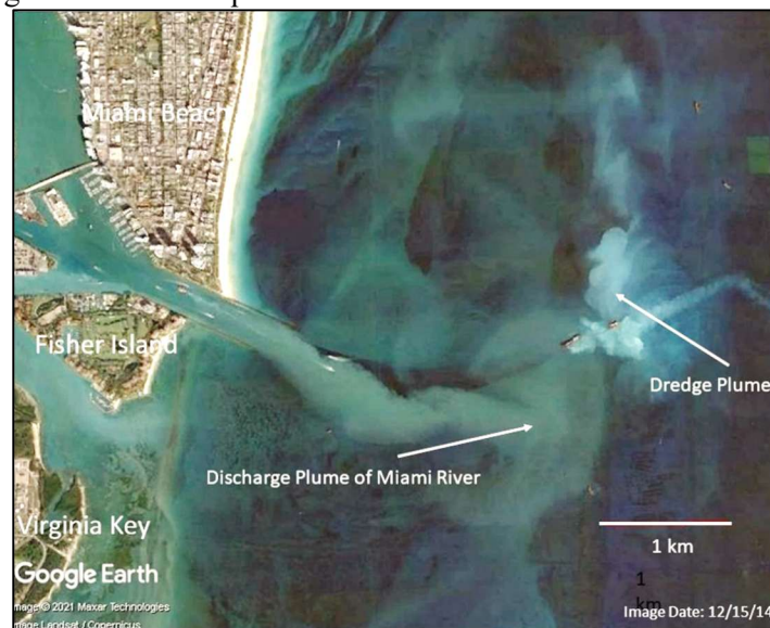
Figure 2. Google Earth Pro Image of the shipping channel entrance to Port Miami. (Government Cut). Image taken on December 15, 2014 during active offshore dredge operations. Turbid dredge plume showing highly reflective (white) optical characteristics of suspended carbonate sediments created by cutterhead dredge operations. Note fine-grained sediments being transported to the north by the prevailing currents. Also note the large plume of turbid water being discharged through the inlet between Miami Beach and Fisher Island. This plume includes a mixture of sediment-laden, nutrient-rich, and highly polluted discharge of the Miami River into the Atlantic Ocean.
