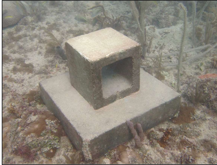
Figure 8. Underwater photo of deployed sediment accumulation block attached to exposed hardbottom. Photo taken on November 12, 2014 during active dredge operations. A colony of the large star coral, Montastraea cavernosa can be seen in the upper left corner of photograph. Note dusting (< 1 mm) of fine sediment deposited on the upper surface of both the block and slab. Photo by RF.
